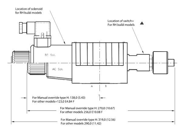
$\blacktriangle$  For LH models ("L" in model code location)  $\boxed{4}$  solenoid and switch locations are reversed riangle Wiring: See warning note on page 5
