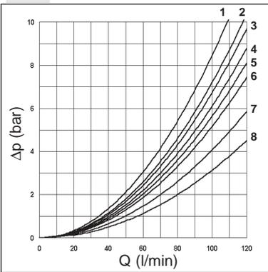
The diagram at the side shows the pressure drop curves for spools during normal usage. The fluid used is a mineral oil with a viscosity of  $46\text{ mm}^2/\text{s}$  at  $40^\circ\text{C}$ ; the tests have been carried out at a fluid temperature of  $40^\circ\text{C}$ . For higher flow rates than those in the diagram, the losses will be those expressed by the following formula:
